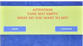
If oil is detected in the tanks, a window appears that allows us or to return to the main menu (HOME), to then reset the value read in the tanks, or to continue the automatic cycle (CONTINUED)
