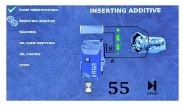
After identifying the flow, the machine will introduce the washing additive previously poured into the special bottle.
