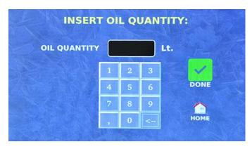
Enter the total amount of oil contained in the gearbox and press (DONE)
