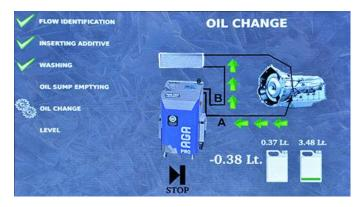
The oil change begins; stay inside the vehicle during this phase and switch the engine on and off as indicated by the green light.
